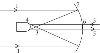
A parallel beam of light 1-1 from a distant natural source, such as the Sun, or from a powerful artificial source installed in the focus of the optical device is directed to the surface of a long-focus concave hyperbolic mirror 2. According to the laws of ray optics, the light beam is collected in the focus 3 of this mirror, which coincides with the focus of another, short-focus hyperbolic mirror (hyperboloid) 4.
