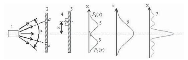
The beam passes through a thin metal plate 2 with two small holes a and b. Behind it there is another plate 3, which absorbs electrons. In front of the plate 3 at a distance x from its axis a detector 4 is suspended, such as a Geiger counter, which counts the number of electrons caught in it. By moving the detector along the plate 3 and counting the number of electrons P(x) per unit time for different values of x, the curves are plotted:
