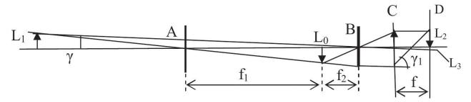
The figure shows that for a telescope it is not the linear but the angular magnification that matters. Indeed, the magnification N of the tube used as a telescope can be calculated as follows.
