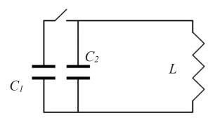
**Problem 117.** In the oscillating circuit, capacitor  $C_1$  is charged to voltage U, and capacitor  $C_2$  is not charged (see figure). The capacitances of the capacitors are equal to each other and equal to C. Ignoring the resistance of the coil L, find the amplitude of the alternating current  $I_m$  arising in the coil conductor after the key is closed.
