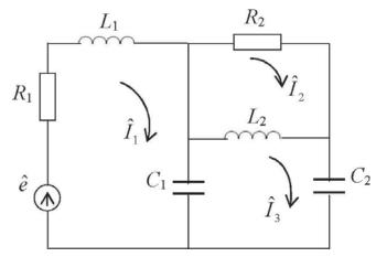
**Solution**. Let us apply the method of mesh currents. The equations for mesh currents in complex form are
